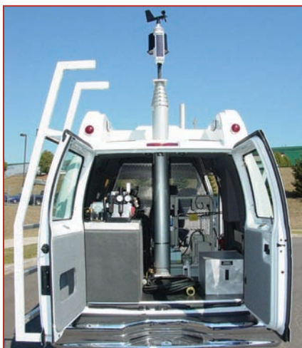
MOVERS (Mobile Vehicle-based Emergency Radiation Monitoring System) is a fully integrated system of radiation monitors and software that can be on the road within minutes to provide real-time radiation survey information.
