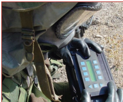
The RAZOR instrument is a hand-portable, identifier designed to move pathogen detection closer to the crisis. Its small, field-hardened design and simple sample preparation makes it the ideal instrument for pathogen detection for military, security & homeland defense personnel.
