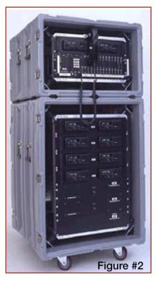
ACU 1000 but also five VHF and five UHF radios. Figure #2 shows the TRP/ACU 1000 in a mobile configuration, and mounted in shock-resistant cabinets; and Figure #3 shows a fixed-site configuration, similar to that used, for example, in a county emergency management center.
